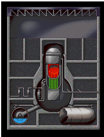
Core Damaged but retained in vessel
